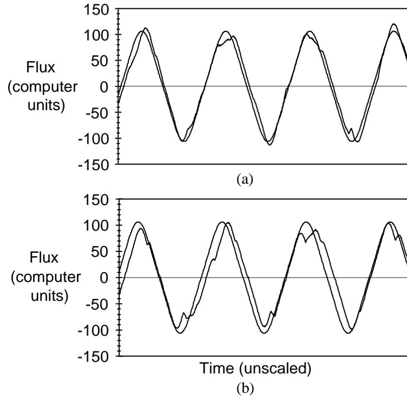
Figure 5.19 Feedback and reference flux waveforms at 26 Hz at (a) no load, (b) full load.
