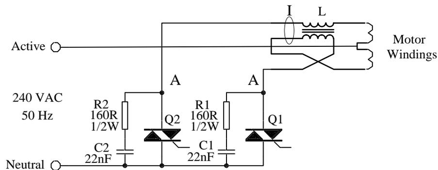
Figure 4.10 Addition of an extra inductor,  $L$ , to increase the effective motor leakage inductance. Nodes AA are the measurement points for phase voltage measurements and loop I shows the current probe connection to measure total phase current.
