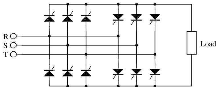
Figure 1.6 Three phase input, 6-pulse cycloconverter.
