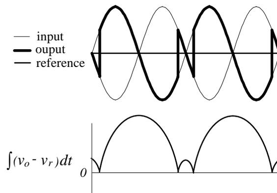
Figure 1.12 An example of instability for a 2-pulse cycloconverter with integral control.
