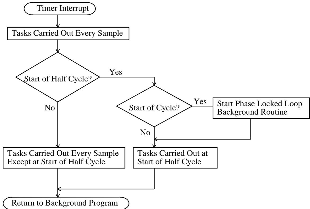
Figure 4.8 Flow chart of the sample routine.
