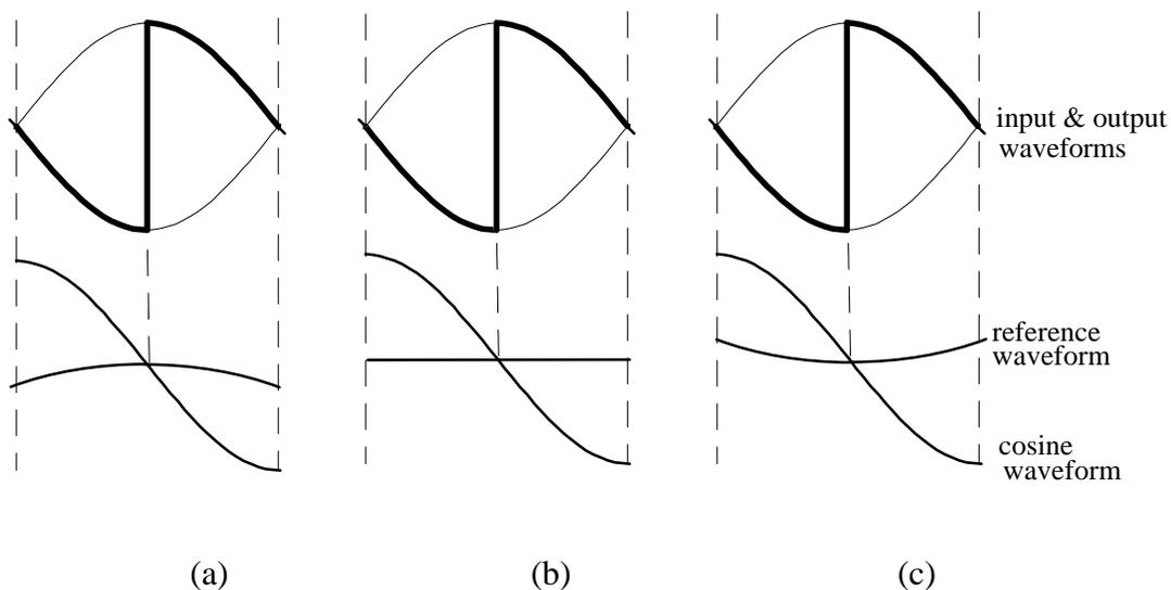
Figure 3.1. Examples of waveforms showing the inaccuracies of cosine wave crossing control. The different reference waveforms with different average levels produce the same output waveforms.
