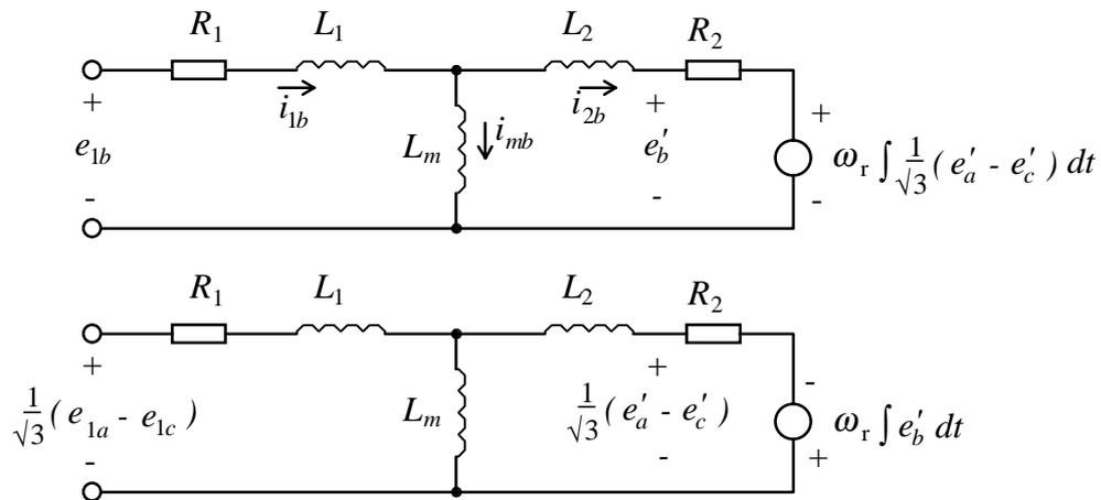
Figure 2.9 Two phase equivalent circuit with transformed variables. The  $\alpha$  axis is aligned with the  $b$  phase.
