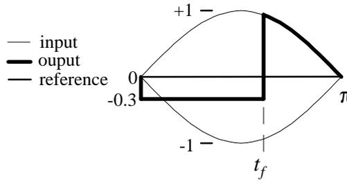
Figure 3.6 Waveforms used for the simulation for determining the stability constant,  $K$ , for the case of discontinuous current.
