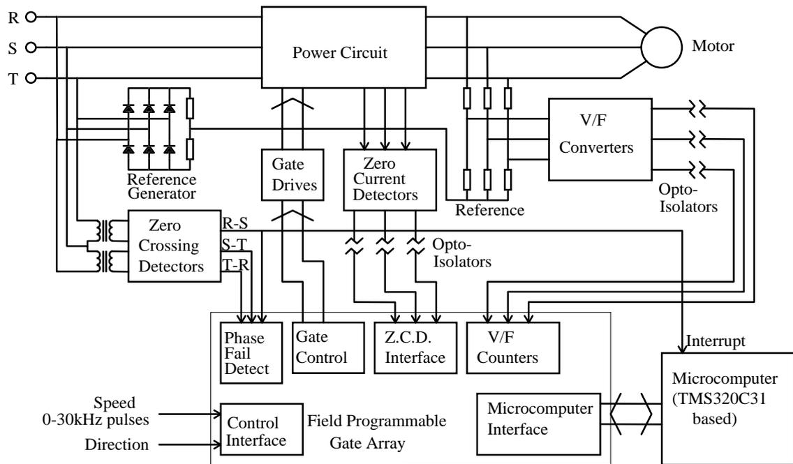
Figure 5.2 Block diagram of the control circuit of the 3-pulse cycloconverter.
