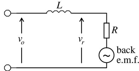
Figure 3.7 Per phase high frequency equivalent circuit of an induction motor with values of the cycloconverter output and reference voltages shown.
