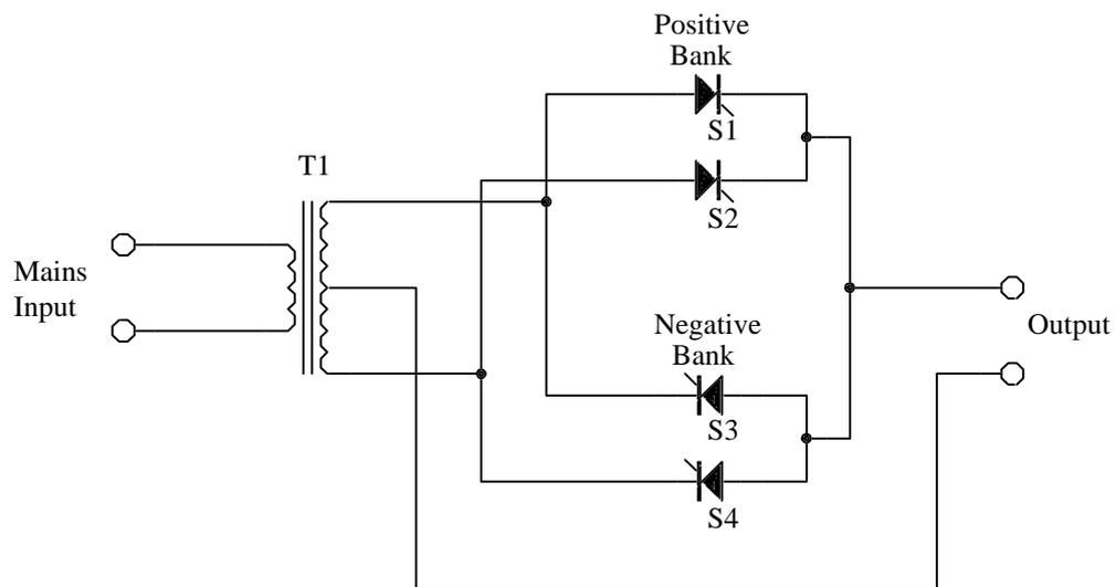
Figure 1.1 Basic single phase cycloconverter.
