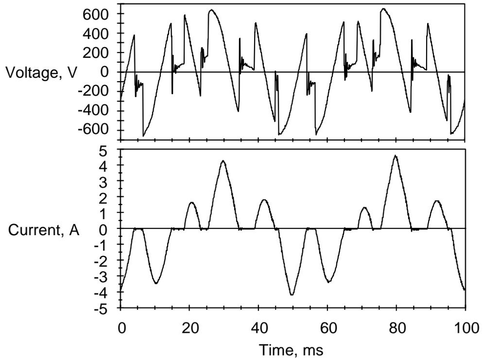
Figure 4.18 Output waveforms for one phase of the 1 to 2 phase cycloconverter operating at 20 Hz with a motor load of 1.4 Nm.
