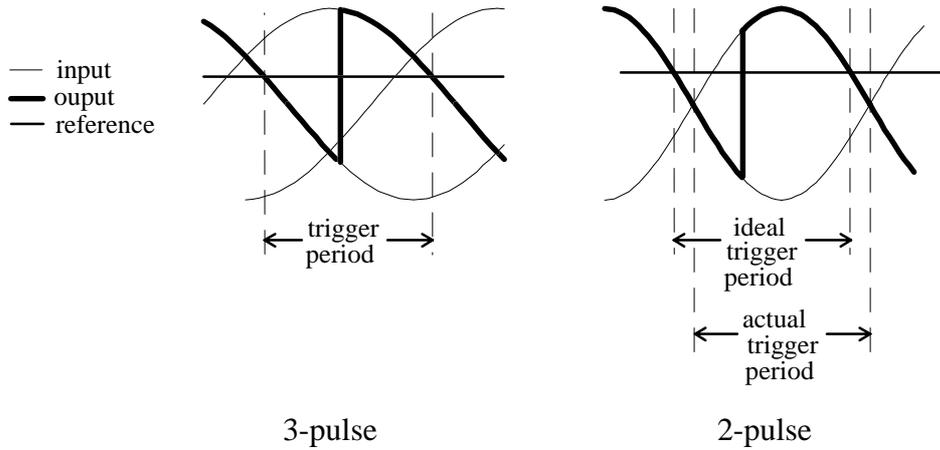
Figure 3.3 Trigger periods for 3-pulse and 2-pulse cycloconverters used for double integral control.
