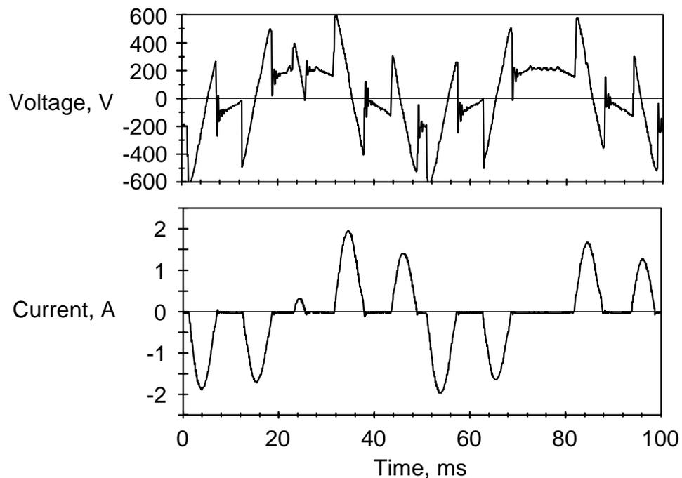
Figure 4.12 Output voltage and current waveforms for one motor phase of the 2 phase cycloconverter at 20 Hz with no load.
