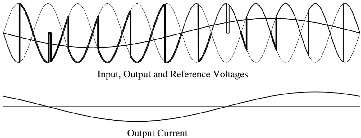
Figure 1.2 Idealised waveforms for a 2-pulse cycloconverter with  $45^\circ$  lagging load current.
