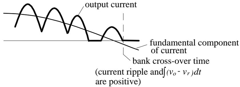
Figure 3.8 Illustration of bank cross-over selection time for the positive bank. Output current must be zero and the integral of  $v_o - v_r$  must be positive.
