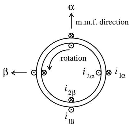
Figure 2.1 Basic two phase induction motor.
