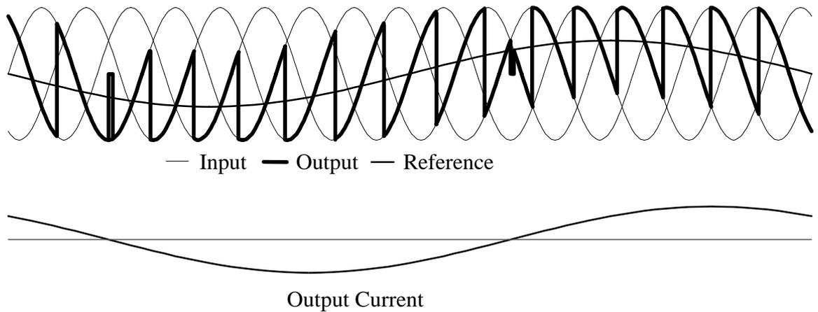
Figure 1.5 Idealised waveforms for a 3-pulse cycloconverter with  $45^\circ$  lagging load current.
