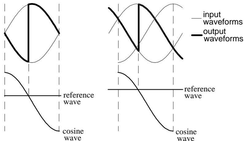
(a) Two-pulse cycloconverter (b) Three pulse-cycloconverter
