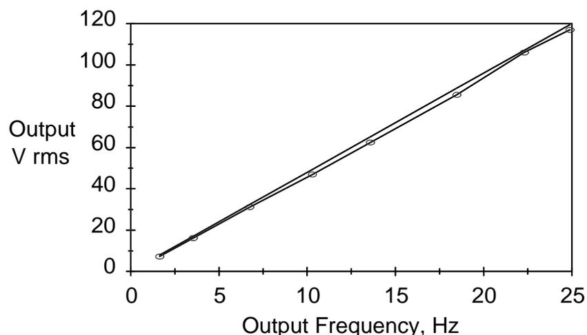
Figure 4.15 Fundamental component of output voltage against output frequency with the ideal straight line value included for comparison.
