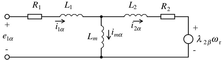
Figure 2.3 Equivalent circuit for the  $\alpha$  phase.
