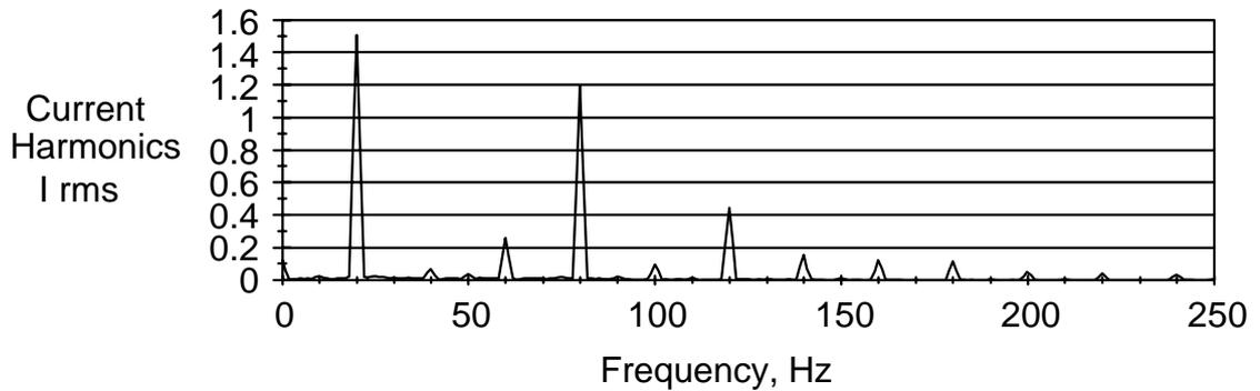
Figure 4.19 Frequency spectrum of the output current with 20 Hz output frequency.
