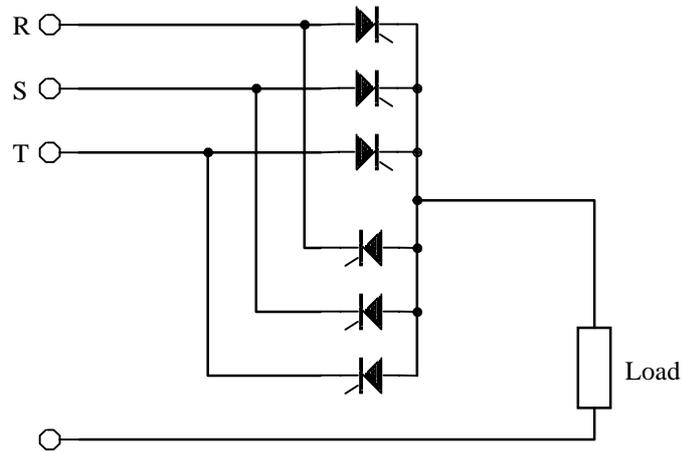
Figure 1.4 Three phase, 3-pulse cycloconverter.
