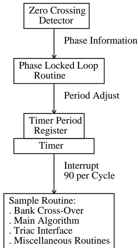
Figure 4.3 Block diagram of the software.
